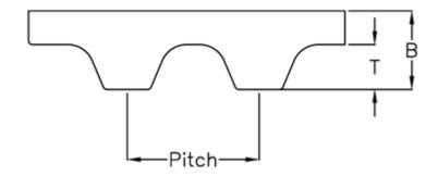
Height B mm= 2.2Height T mm= 1.2Length= 650Number of teeth= 130Pitch= 5Type= PU 25 T5 650Width= 25
